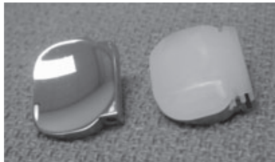
Figure 8. The PCM ® artificial spinal disc prosthesis (PCM-040) after 10 million cycles.
