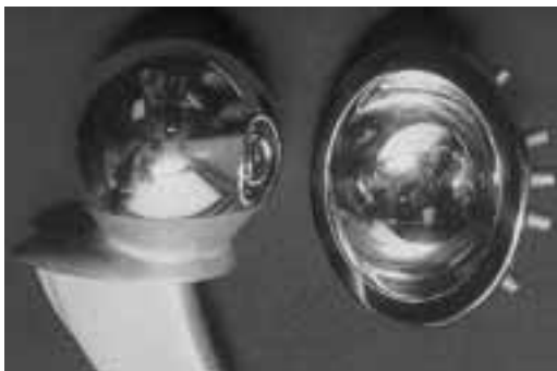
Figure 6: McKee-Farrar metal-metal implant retrieved after 25 years in situ. From: Chan, et al., AAOS Scientific Exhibit , 1997.
