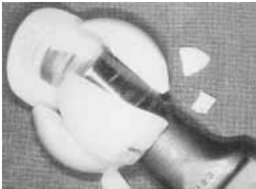
Figure 5: Fracture of an Alumina ceramic ball 6 years after implantation. From: Wagner, Sem in Arthro 9:143, 1998.
