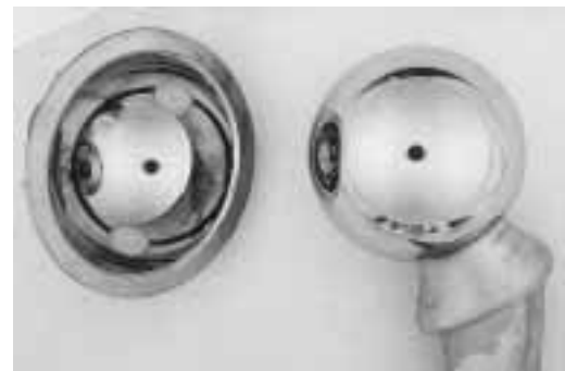
Figure 7: Müller metal-metal implant retrieved after 20 years in situ. From: Wagner, Sem in Arthro 9:143, 1998.
