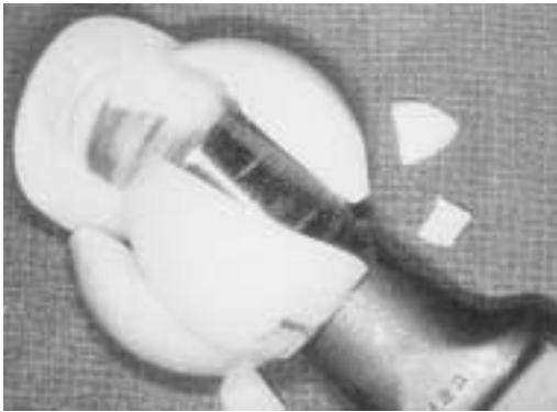
Figure 5: Fracture of an Alumina ceramic ball six years after implantation. From: Wagner, Sem in Arthro 9:143, 1998.
