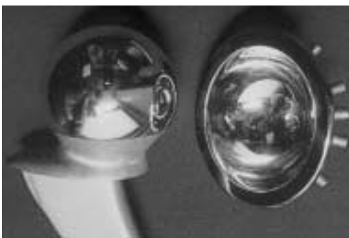
Figure 6: McKee-Farrar metal-metal retrieval after 25 years in situ. From: Chan et al., AAOS Scientific Exhibit , 1997.
