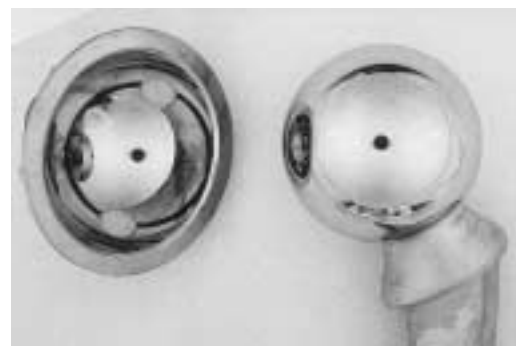
Figure 7: Muller metal-metal retrieval after 20 years in situ. From: Wagner, Sem in Arthro 9:143, 1998.
