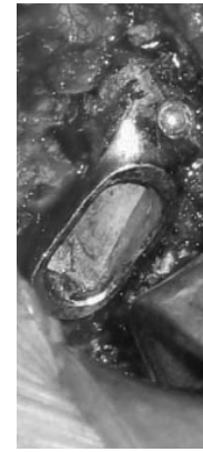
A clinical example where fretting and corrosion are visible on the stem/neck junction.
