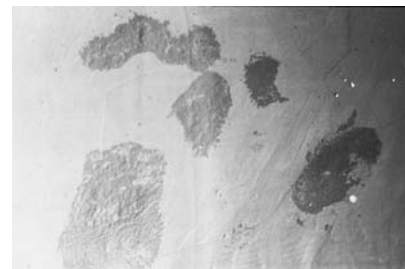
SEM displaying material loss on a metal-metal taper interface resulting from fretting (x15 magnification)
