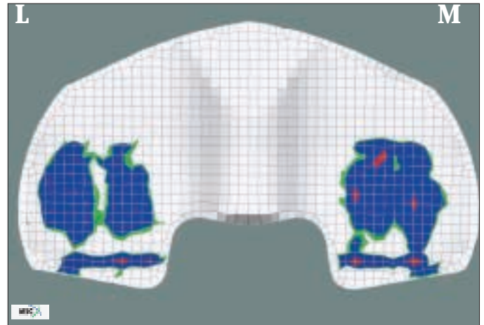
Midstance: 2.0 BW, 20° flexion Contact Area: 476 mm 2
