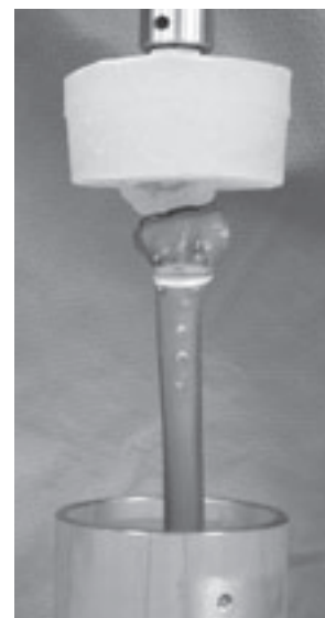
Figure 4: Plate-synthetic composite bone construct on MTS. Note osteotomy and beads for measurements.
