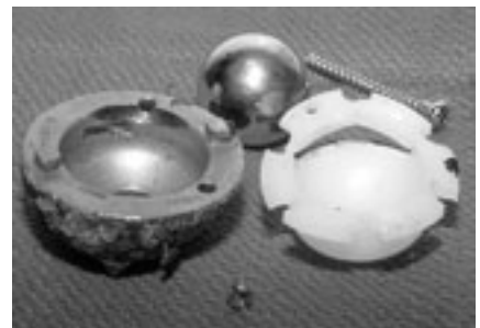
Figure 12: Crack propagation failure of a retrieved conventional polyethylene liner associated with an inadequate locking mechanism design.
