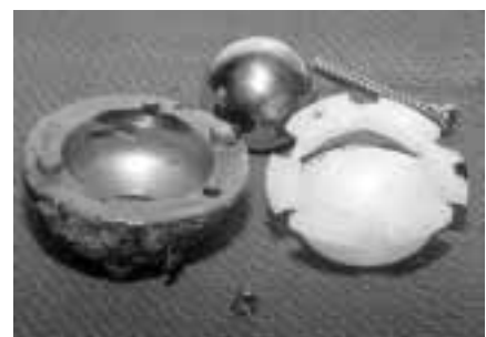
Figure 12: Crack propagation failure of a retrieved acetabular cup associated with an inadequate locking-mechanism design.
