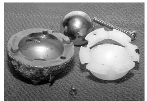
Figure 7: Crack propagation failure of a retrieved conventional UHMWPE liner associated with an inadequate locking mechanism design.
