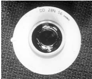
Figure 11: A failed Hylamer acetabular cup insert retrieved 3 years after implantation.
