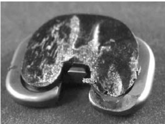
Figure 10: A failed Poly-2 tibial insert retrieved 5 years after implantation.
