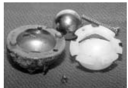
Figure 12: Crack propagation failure of an acetabular cup retrieval that is associated with an inadequate locking mechanism design.
