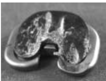
Figure 6: Five-year retrieval of a failed Poly-2 tibial insert.
