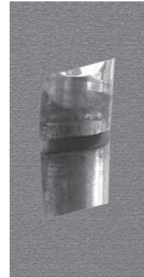
A close-up view of a fretting-induced fracture site for the ProFemur
