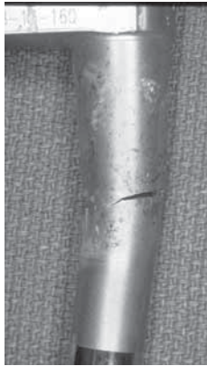
A close-up view of a fretting-induced fracture site for the S-ROM
