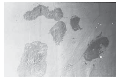
Scanning Electron Microscopy (SEM) displaying material loss on a metal-metal taper interface resulting from cyclic microdisplacements (x15 magnification)
