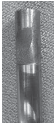
A close-up view of a fretting surface for the Link MP
