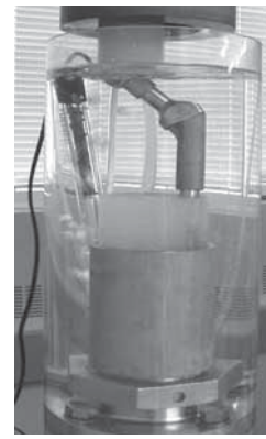
For this particular example of the Link MP, the level of potting approximates the distal end of the taper to appreciate its structural integrity
