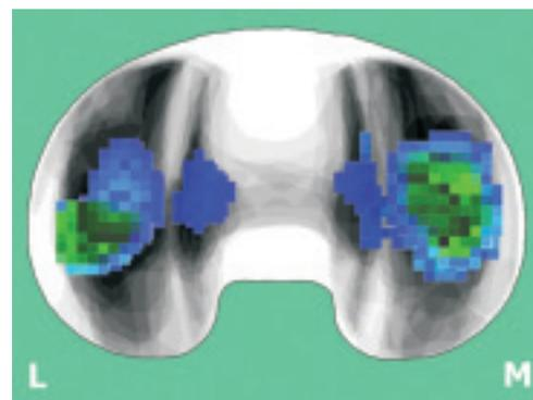
Figure 3: Retrieval wear scar pattern with KneeSIM overlay of accumulated pathways of contact stress.
