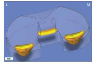
of identical stress magnitude, and when present, appear as concentric ellipsoids or cylinders. They represent a visual inference
