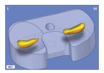
background) give an indication of the areas where surface abrasion caused by contact with the femoral component can occur. The
