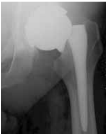
CASE 1 - A clinical example of a modular femoral neck, titanium alloy, primary system. Device fracture is observed at the neck/stem junction two months after a fall. This device survived in situ in this 340 lb patient 4 years before the trauma. The view of the stem/neck junction describes fretting and corrosion at the interface. 22
