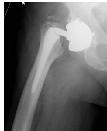
CASE 2 – A clinical example of a modular femoral neck, titanium alloy, primary system. Device fracture is observed at the neck/stem junction. A long varus neck coupled with a BMI of 34.2 and moderate activity contributed to device failure at 29 months in situ.
