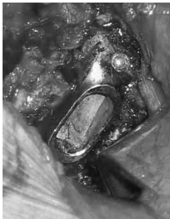
CASE 1 - A clinical example of a modular femoral neck, titanium alloy, primary system. Device fracture is observed at the neck/stem junction two months after a fall. This device survived in situ in this 340 lb patient 4 years before the trauma. The view of the stem/neck junction describes fretting and corrosion at the interface. 22
