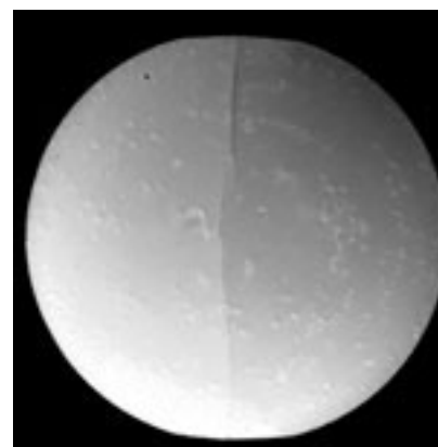
Classic Diametral Tension Fracture
